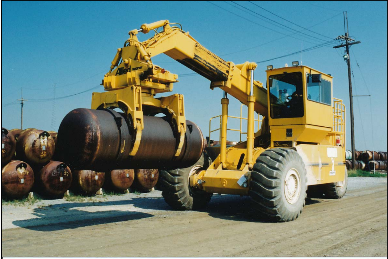
Figure 6-11. A specialized hoist is used to move one of the approximately 46,000 canisters containing depleted uranium hexafluoride (DUF6) stored at the PDGP.
