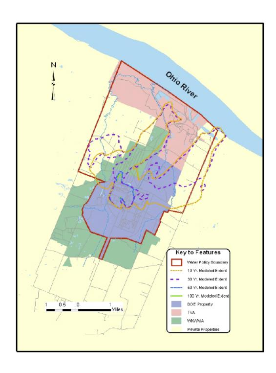
Figure 3.5.4 Predicted TCE Plume Contours (5  $\mu$ g/L) Over Time Assuming Source Reductions at C400, C720, SWMU1 and SWMU4 (including dissolved phase treatment of Southwest Plume and PTZ at facility fence) (Scenario 4)
