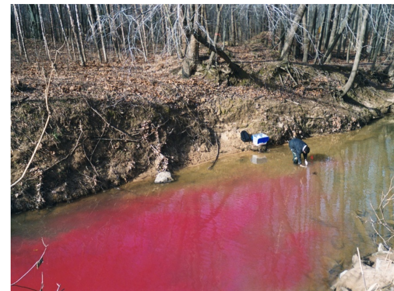
Fig. 3. Approach of tracer cloud to first sampling point (LBC-3B), January 2003.
