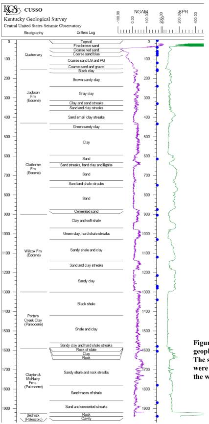
Figure 3. Stratigraphic and geophysical well log interpretations. The stratigraphic interpretations were made from cuttings collected at the well head.
