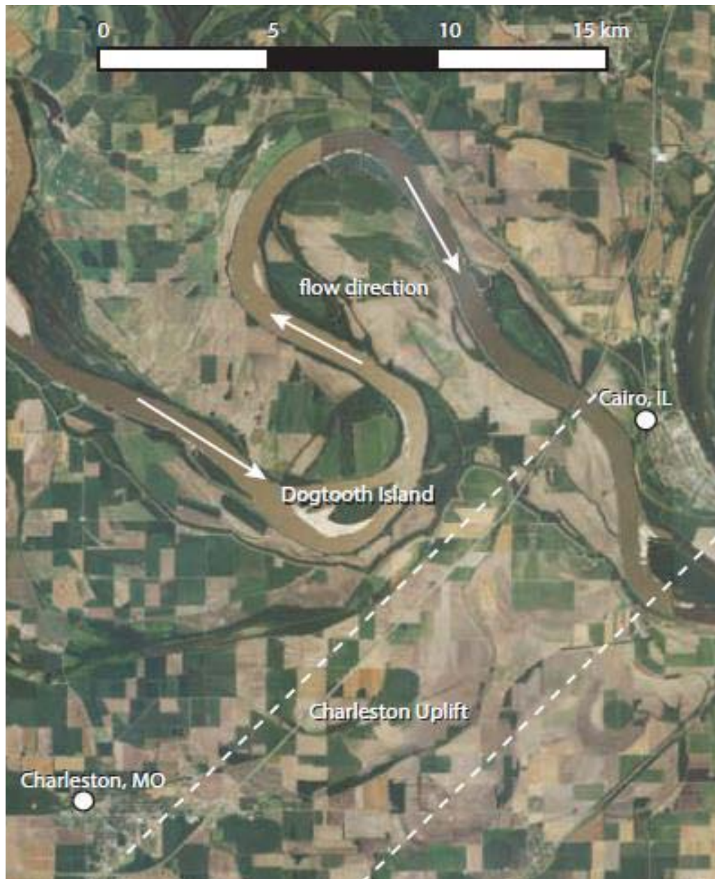
Figure 8. A closer view of the Pyrne et al. (2013) projection of the Charleston uplift crossing the Mississippi River near Cairo, Illinois. The intersection is marked by a meander that changes 180 degrees and flows up valley for nearly 10 km in order to get around the Charleston uplift. This geomorphic signature is similar to the torturous meander in the river (the Kentucky Bend) at New Madrid, Mo., where it changes flow direction 180 degrees and flows up valley for approximately 15 km in order to get around the Tiptonville dome/Lake County uplift (Van Arsdale et al., 1995).
