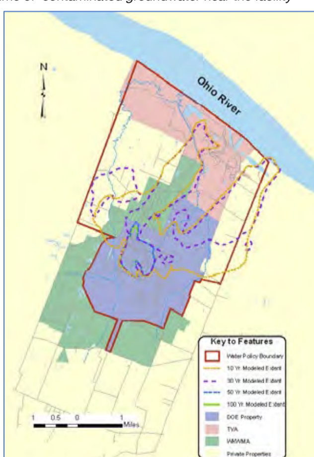
Modeled maximum TCE Plume Contours at 500 µg/L over time assuming Source Reductions at C400, C720, SWMU1 and SWMU4 (including dissolved phase treatment of Southwest Plume and PTZ at facility fence) (Scenario 4)
