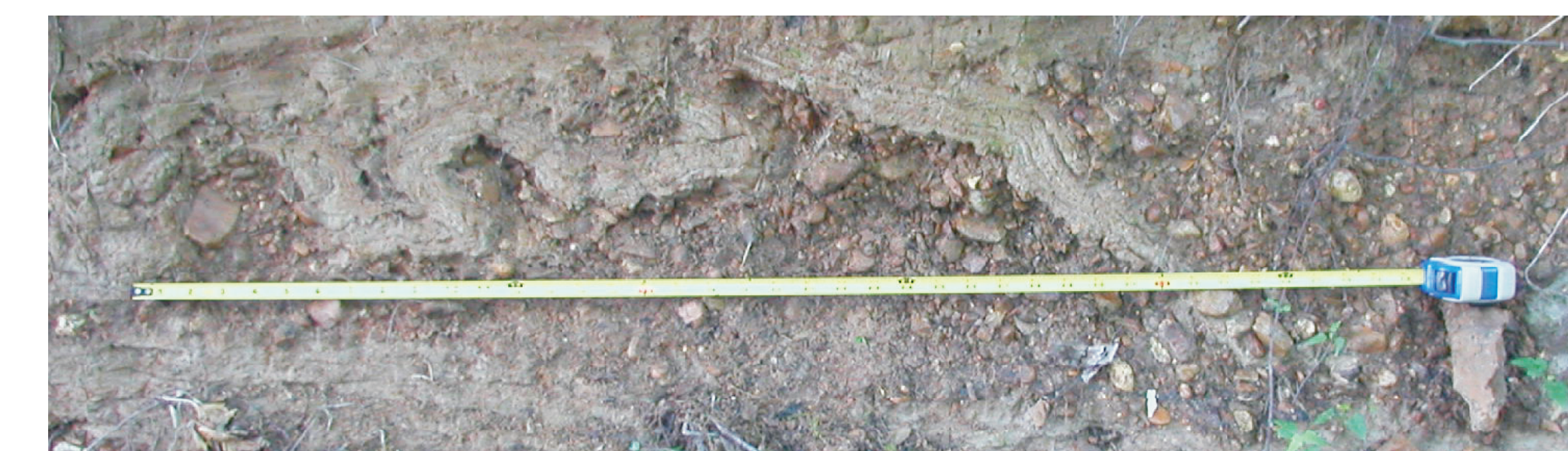
Image 4: Paleo-liquefaction feature noted along Bayou Creek
